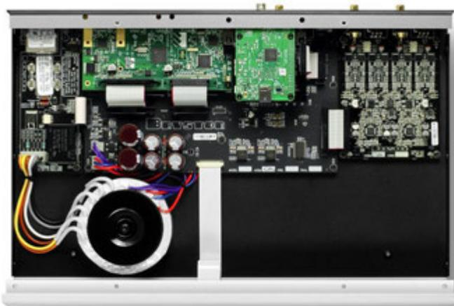
Bryston BDA-3.14 is a streaming player that was created by connecting the BDA-3 digital-to-analog converter with a network module based on the Raspberry Pi platform, previously used in BDP-Pi transport. Both sections are connected by the I<sup>2</sup>S bus, which - as we read on the manufacturer's website - is currently the most accurate method of sending a digital signal.
