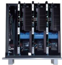
**Modular design with independent power supplies each with its own transformer for precise sound-staging.**
