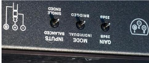
*On the back of the Bryston 3B<sup>3</sup> are toggle switch to select the gain, the mono-bridged or stereo operation and the input selection*
