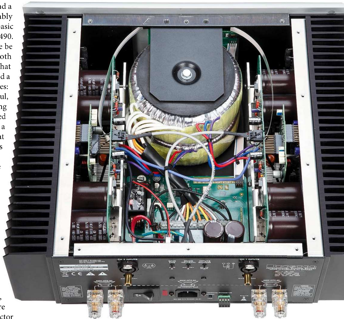
▲ Two stacked and solidly clamped toroidal core transformers contribute to the hefty weight of the 4B3.
