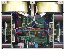
the source that over the mains current no harmful RF components can get into the circuit. Speaking of mains power: Instead of - as often happens - a transformer with two taps, the Bryston 3B³ were two separate toroidal transformers, for each channel one, donated. Sophisticated, solid technology, of course, always pleases the tester's heart - but what does the whole thing do in the listening room?
