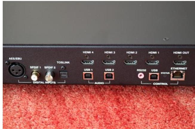
The BDA-3 can decode PCM up to 384kHz/32 bit and up to DSD-256, through asynchronous USB inputs, and accepts both PCM and SACD input via HDMI. As it does not decode surround formats, the BDA-3 will use EDID for handshaking between devices to only retrieve 2 channel material from a disc. Although it does not process surround sound, the BDA-3 can actually pass through the incoming signals to another receiver such as a surround processor or a display, provided that a non-HDMI input is selected.
