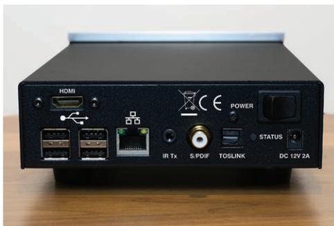
Bryston's BDP- $\pi$  digital music player has four USB ports for connecting external drives and output to a USB DAC. There are also TOSLINK optical and SPDIF coaxial digital outputs, plus HDMI. The USB, TOSLINK and SPDIF outputs support resolution to 24 bits/192kHz; HDMI is limited to 16/48.
