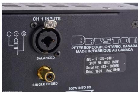
Bryston are absolute minimum values and are regularly exceeded in practice. Our Bryston 4B3 amplifier with a specified 300 Watts into 8 ohms, actually supplied 332 Watts according to our measurements, and in bridged mode which is rated at a nominal 900 watts, it actually supplied 1080 Watts.
