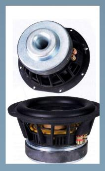
Here many a PA and CarHiFi chassis should go green with envy: The bulbous rubber surround is optimized for the highest excursion, the large voice coil on cardboard is substantially vented by being rear ventilated and by holes in the pole pieces, and made immune from compression.
