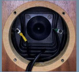
The midrange speaker is located in a closed plastic compartment with airtight terminals, whose shape is stepwise constricted for suppression of standing waves. The small midrange cone is a recognizable midrange specialist, beside the strong magnet everything is optimized for lightweight construction and fast impulse processing, even the speaker die cast basket is made from aluminum.
