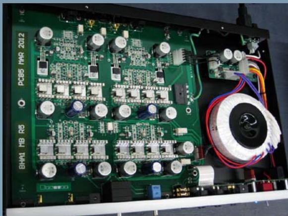
The circuitry of the BHA-1 Headphone Amplifier consists primarily of six discretely built-up (with individual transistors) operational amplifiers, of which two serve as input amplifiers (above), and the other four in channel connected pairs as bridged amplifiers (below). The analog operating loudness potentiometer from Noble (little blue box) follows in the signal path after the balanced input stage.
